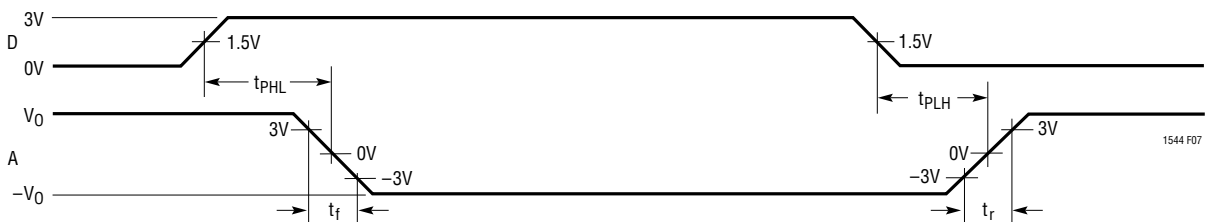
Figure 7. V.10, V.28 Driver Propagation Delays
